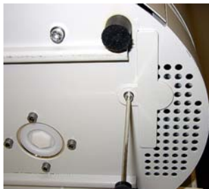
Fig. 46: Loosening the air filter cover
