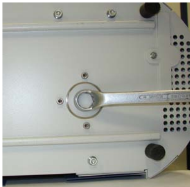
Fig. 48: Fastener of the operating fluid reservoir
