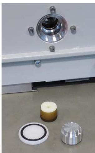
Fig. 49: Opened operating fluid reservoir
