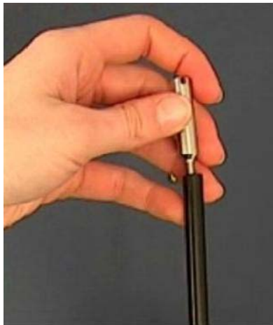
Fig. 8: Tightening the water conservation sniffer probe
