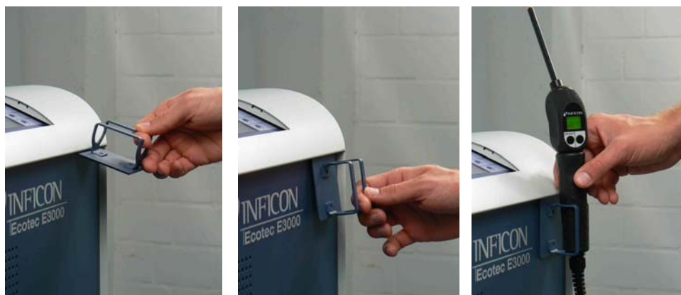
Fig. 9: Sniffer line holder mounting
