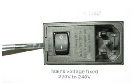
Fig. 51: Levering out cover to the right
