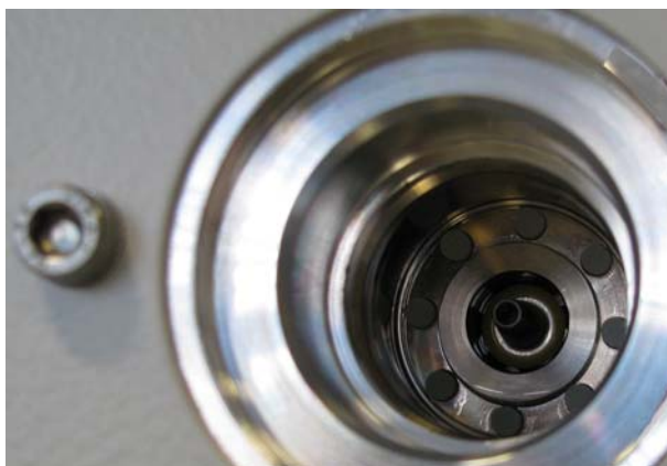
Fig. 50: Porex rods of the operating fluid reservoir
