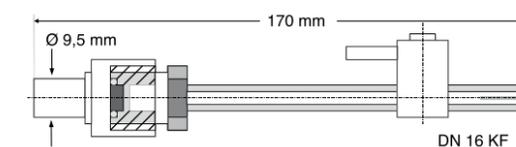
Calibrated leak with pin type casing and VCO fitting
