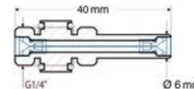
Calibrated screw-in leak
