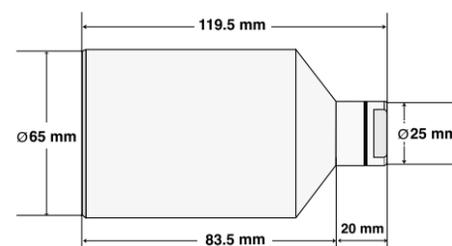
CONTURA Z integral test leak
